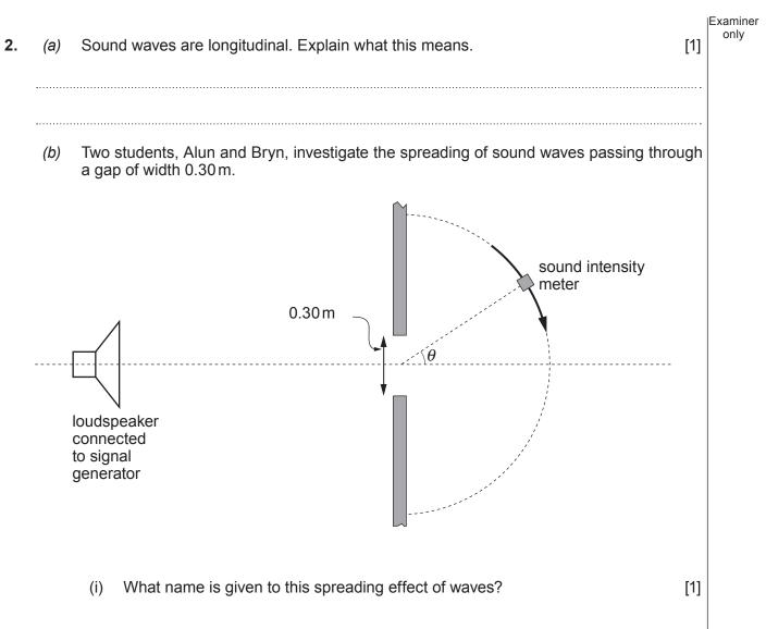
(ii) Alun moves a sound-intensity meter around the semicircular path shown opposite, taking readings at various angles,  $\theta$ . The graph below shows the results.
